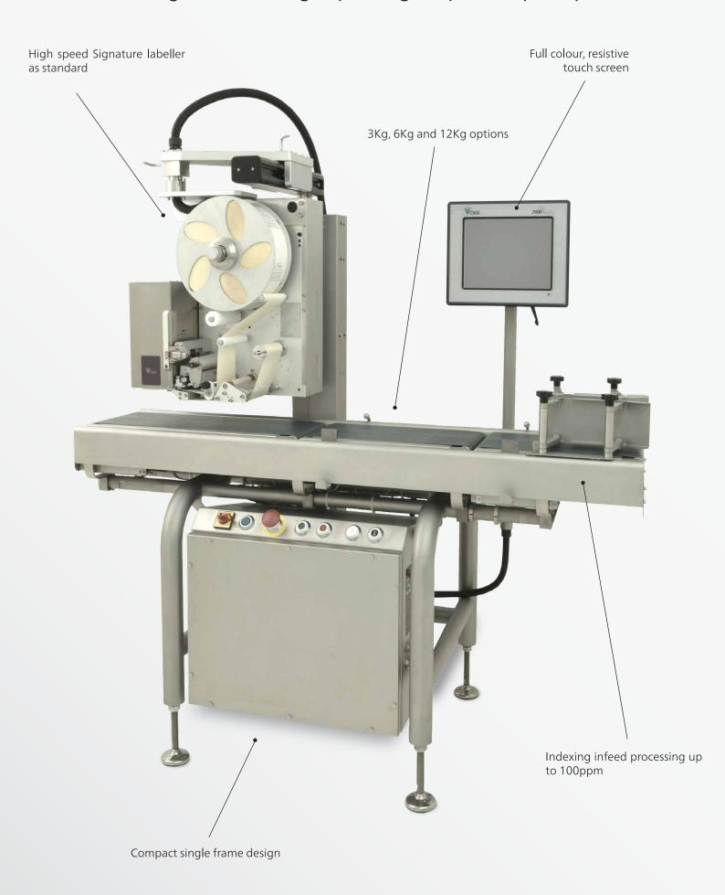
The MI-700 is designed to be compatible with a variety of DIGI labellers, printers, conveyors, guides and rejectors as well as external devices such as metal detectors, sleevers, scanners and wrappers.
